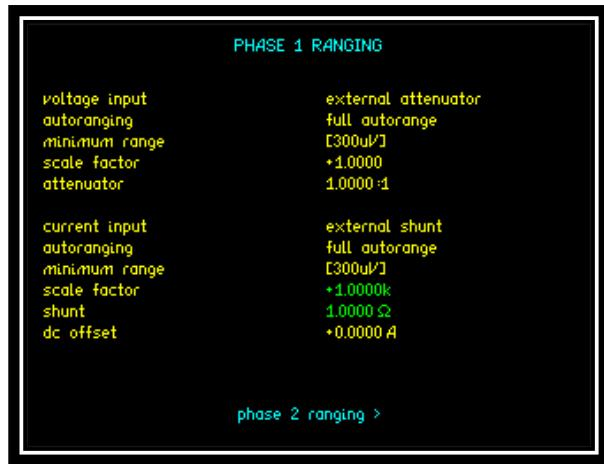
Only the settings stored in program location 1 are automatically recalled each time the instrument is switched on. Should it be preferred to not have them automatically recalled they can instead be saved to an alternative memory location and then deleted from location 1. The User can then recall the System Calibration data when required. The Program Store/Recall/Delete menu should be used to make the changes:
