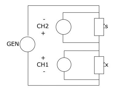
For "shunt" connection, shown above, the current is measured directly across the shunt using CH2 while the voltage across the Zx is measured by CH1. Notice that the positive inputs to both CH1 and CH2 are connected to the midpoint to minimise common mode loading effects.
