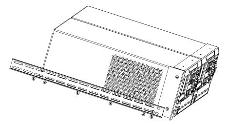
5. Fix the right fixing part to the right side of the front panel of instrument B using two M4 screws.
