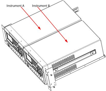
6. Fix the other rack rail at the right side of the rack support shelf using seven M4 screws.
