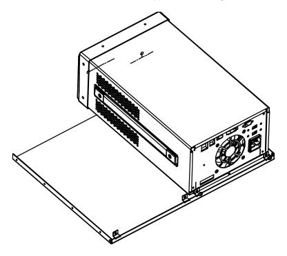
3. Fix the left fixing part at the left side of the front panel of the instrument using two M4 screws.
