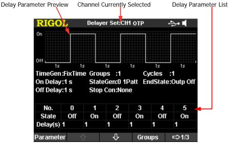
Figure 2-4 Delay Parameter Setting Interface
