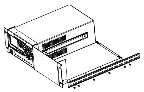
7. Fix the other rack rail at the left side of the rack support shelf using seven M4 screws.
