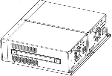
3. Fix the left fixing part at the left side of the front panel of instrument A using two M4 screws.
