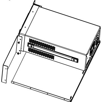
5. Fix the right fixing part to the right side of the front filler panel using two M4 screws.
