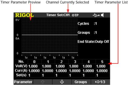
Figure 2-2 Timer Parameter Setting Interface
