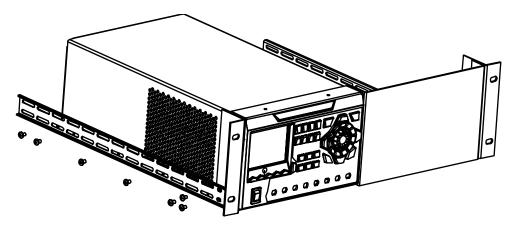
8. Fix the two side beam fixing parts to the end parts of the left and right rack rails respectively using four M4 screws.
