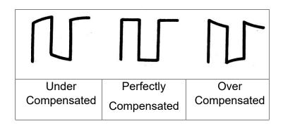
Use a non-metallic screwdriver to adjust the low-frequency compensation adjustment point on the probe until the waveform displayed matches the "Perfectly compensated" example.
