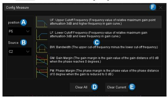
A. Set the position of measurement items, and support 5 measurement items at most
