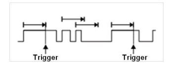
Trigger source, slope (rising, falling), dropout type and time value can be set in the trigger dialog box. Holdoff, coupling and noise reject can be set in dropout trigger, see the sections " Holdoff", " Trigger Coupling" and " Noise Reject" for details.
