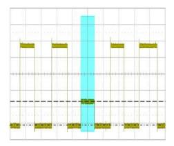
First, set the trigger type to Runt, in order to trigger on the dwarf pulse. See the section "Runt Trigger" for details.
