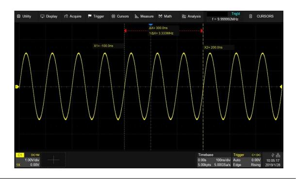
Fixed position, timebase is changed to 100ns/div, the grid number of X cursors (-1div, +2div) remains fixed. The value of X1 and X2 are changed to -100ns, 200ns.
