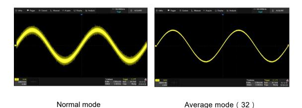
Note: Average acquisition is only valid for periodic signals, and it is important to ensure that the waveform is triggering in a stable way when using average mode.
