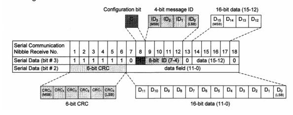
Frame (enhanced serial message with 8bits ID) - 12-bit data and 8-bit message ID, the configuration bit is 0.
