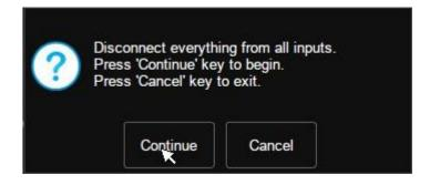
The oscilloscope will not respond to any operation until the self-cal is finished. After the self-cal is completed, touch the screen or press any button to exit.
