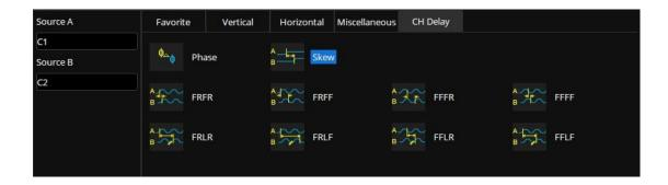
In the parameter selection area, the channel corresponding to Source A is specified first, and then the channel corresponding to Source B. Finally, the measurement parameter is selected. For example, to activate the skew between C1 and C2, you can follow the steps shown below:
