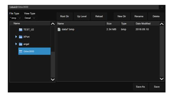
In step 4, if Save is selected instead of Save As, the system saves the file as the default file name t3dso3000 n.bmp, where n is an integer incrementing from 1.
