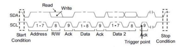
**10 bit Address & Data** - If all bits match, then trigger on the Ack bit followed by the Data.
