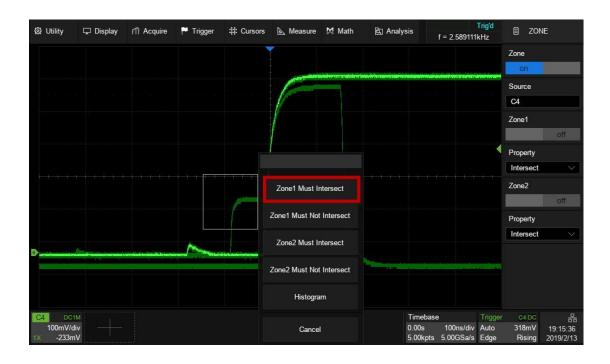
Now, we can accurately capture the exact bus contention waveform:
