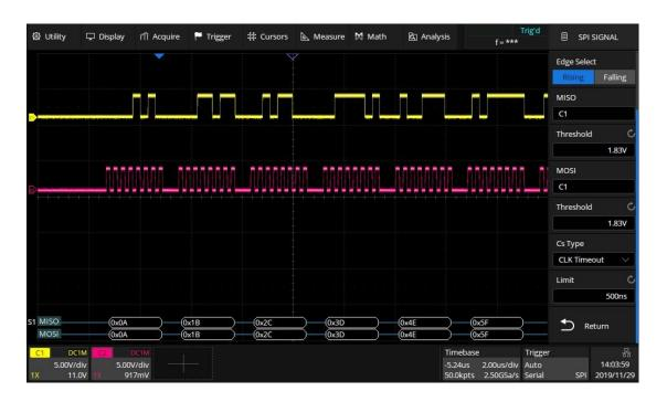
If the data width is set to be greater than 8 bits (such as 16 bits), measure the clock idle time between 8-bit data packets as 0.57 us, and then set the timeout time to a value between 0.57 and 150 us. In this example, it is set to 1 us:
