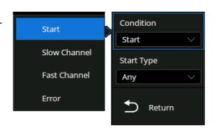
**Start** - the oscilloscope will be triggered on the start of the message (after 56 synchronization ticks). You can select the type of the message: Fast Channel Message, Slow Channel Message or any.
