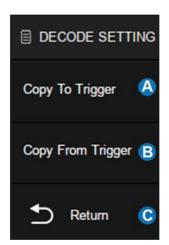
Note: The synchronization is not automatic. If the settings in one place change, a copy operation is necessary to re-synchronize.
