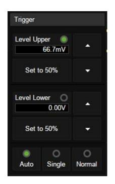
1. Touch the Level Upper area in the quick menu to select the upper level, and then set the level value by the virtual keypad or the Level knob on the front panel. To set the lower level is the similar.
