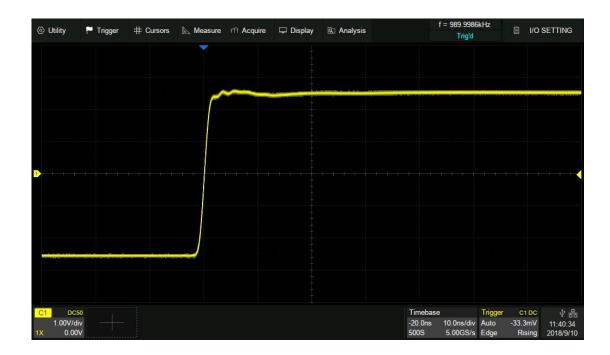
Timebase=10ns/div , Horizontal Delay=-20ns=-2div
