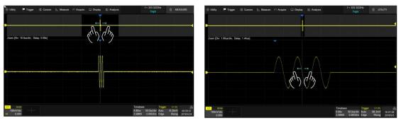
Adjust the horizontal scale of Zoom window by horizontal pinch and spread in the zoom area of the main window or in the Zoom window
