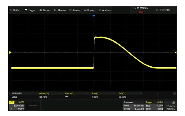
In the example, 53969 pulses can be obtained with the sample rate of 5 GSa/s at the maximum memory depth.
