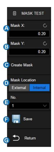
Set the values for Mask X and Mask Y (in divisions of display graticule), and then perform Create Mask to generate the mask. The horizontal and vertical adjustment range is 0.08-4.00 div.
