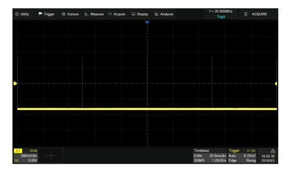
In normal mode, 5 pulses can be obtained on the screen with the sample rate of 1.25 GSa/s at the maximum memory depth.
