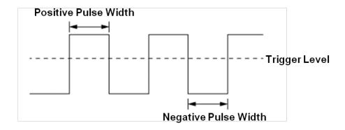
**Less than a time value (≤)** - Trigger when the positive or negative pulse time of the input signal is lower than the specified time value. Below is an example of trigger condition is set to positive pulse width < 100ns
