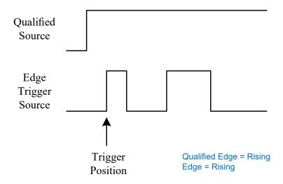
Touch the Qualified Setting region to set the qualified source and threshold; Touch the Edge Setting region to set the edge trigger source, threshold and slope.
