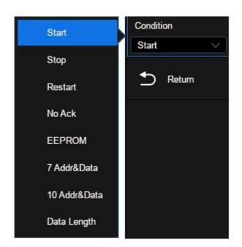
**Start** - The oscilloscope will be triggered when the SDA line transitions from high to low while the SCL is high.
