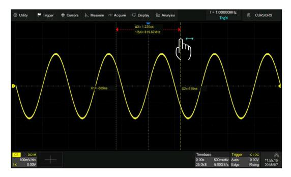
Touch the display area of  $\triangle X$  (or  $\triangle Y$ ) in M1 mode and drag it to move the two cursors simultaneously, as shown in the figure below. This is equivalent to the operation on the cursor type X1-X2 or Y1-Y2.
