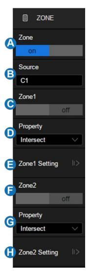
The zones can be created and moved by gestures or by setting Zone > Zone Setting in the dialog box. The color of the zone's outline is consistent with the color of the specified source (Channel 1 = Yellow, etc...).
