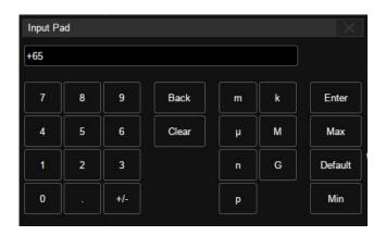
Using the operation of setting the 'deskew' of a channel as an example: If the expected value is 65 ns, input '65' on the virtual keypad, and then choose the unit 'n' to complete the operation. On the virtual keypad, touching the buttons Max, Min, and Default will quickly set the parameter to its maximum, minimum or default value.
