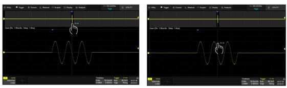
Adjust the horizontal position of the zoom area by dragging left and right in the zoom area of the main window or waveform in Zoom window
