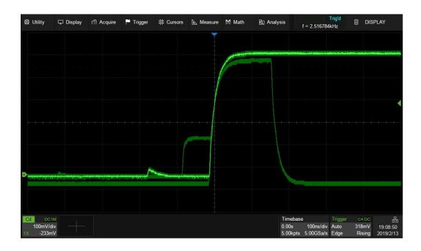
In this case zone trigger is a quick and simple way to capture the interested waveform. Enable the zone trigger, and draw a box to intersect with the bus
