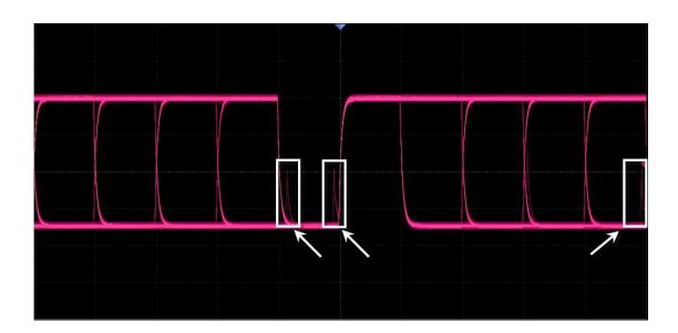
When the display dialog box and persist are off, double pressing the Display/Persist button on the front panel can quickly turn on persist.
