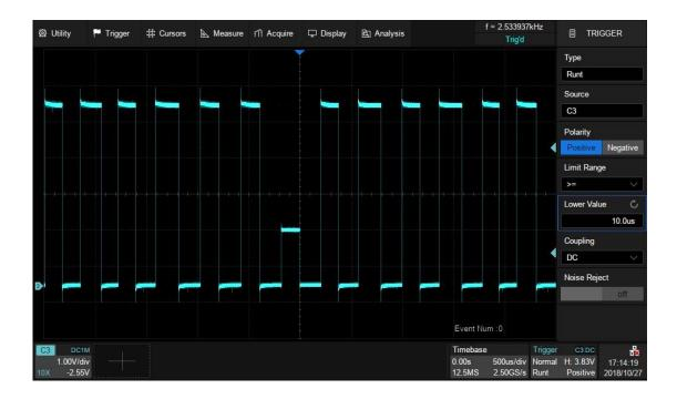
Then turn on Search function and operate Copy from Trigger in the search dialog box so that the oscilloscope searches for the dwarf pulses using the same settings as the trigger.
