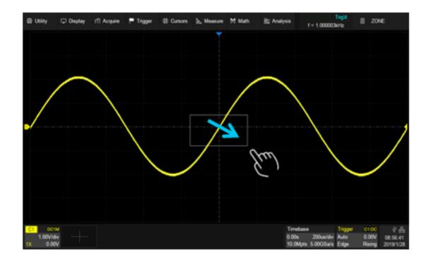
When the finger moves out of the screen, a menu pops up allowing you to select the zone and set the zone properties:
