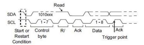
**7 bit Address & Data** - the oscilloscope will be triggered on a read or write frame in 7-bit address mode.
