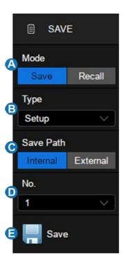
A progress bar is shown when the Save operation is in progress. When it is done, the oscilloscope prompts "Saved to internal file No.X", where X is the internal storage location index selected in the step ①.
