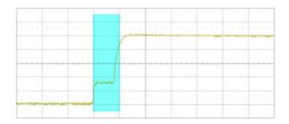
With a simple edge trigger, it is unlikely to trigger consistently on this anomaly. Thanks to the high waveform update rate of the T3DSO3000, we can confirm that bus contention is happening by enabling the persistence display, as shown in the figure below:
