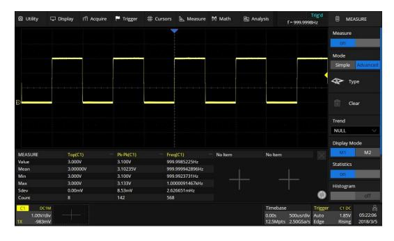
In M2 mode, up to 12 parameter measurements are displayed at a time. When statistics are enabled, they are distributed on the right side of the measurement item. Touch a row to add or replace a measurement.
