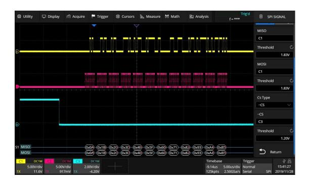
When the CS type is set to Clock Timeout, turn on a Cursor, measure the clock idle time between frames as 150 us, and measure the interval between the clock pulses as 0.14 us, then set the timeout to a value between 0.14 and 150 us. In the example shown below it is set to 500 ns:
