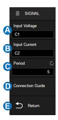
Touch Signal>Connection Guide to recall the connection guide of power quality, as shown in the figure below. Please follow the instructions in this figure for the correct connections. Touch the icon on the top right of the guide to close.
