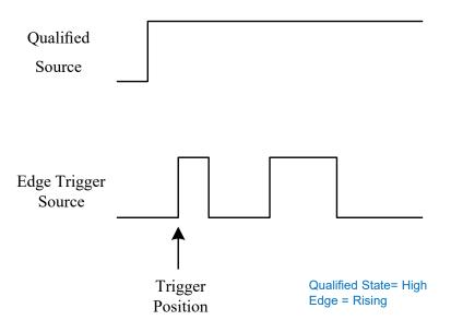
When the type is "Edge", the oscilloscope triggers at the first edge after the specified edge (Rising or Falling) of the qualified source; when the type is "Edge with Delay", time limit condition is available.
